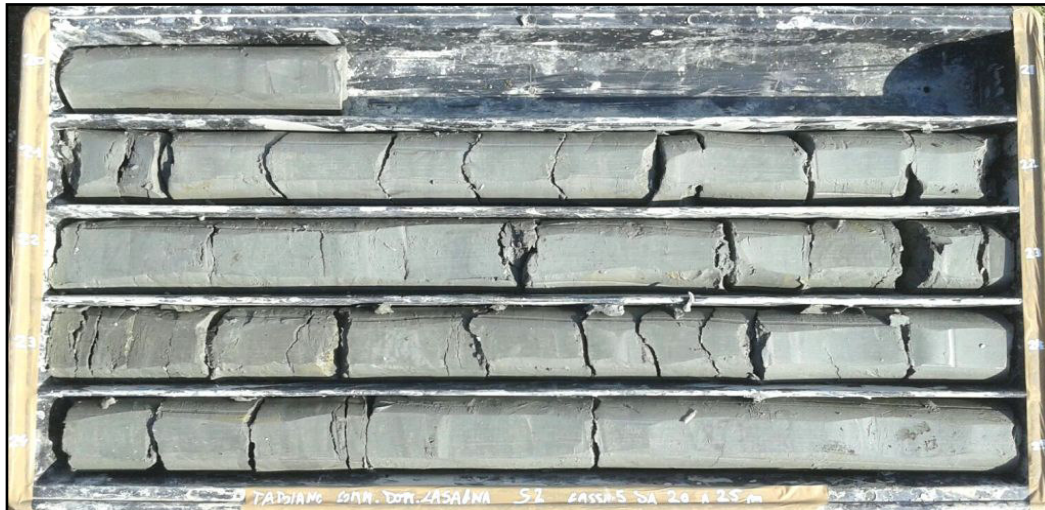
S2 - Cassetta da 20,0 a 25,0 m da p.c.
