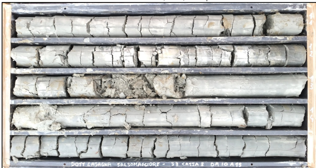
S3 - Cassetta da 10,0 a 15,0 m da p.c.
